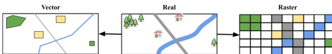
Figure 2.6. Vector and raster structures (Adapted from [Lisboa Filho and lochpe 2001])
