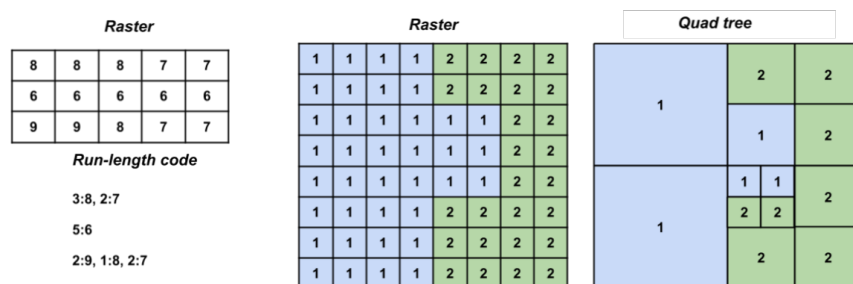
Figure 2.7. Run-length and Quad Tree compression of raster data
