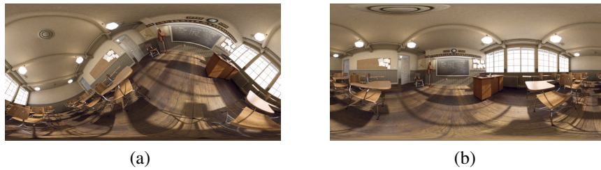
Figura 2.5: A (a) tilted 360^\circ capture (in ERP format) of the same scene as in Figura 2.1b and (b) its upright aligned version using the estimates from the method in [Bergmann et al. 2021].
