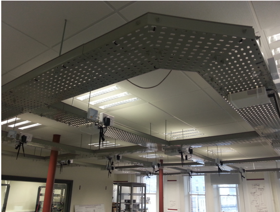
Figure 3.28: Iris wireless laboratory ceiling mounted N210 USRP radio equipment.
