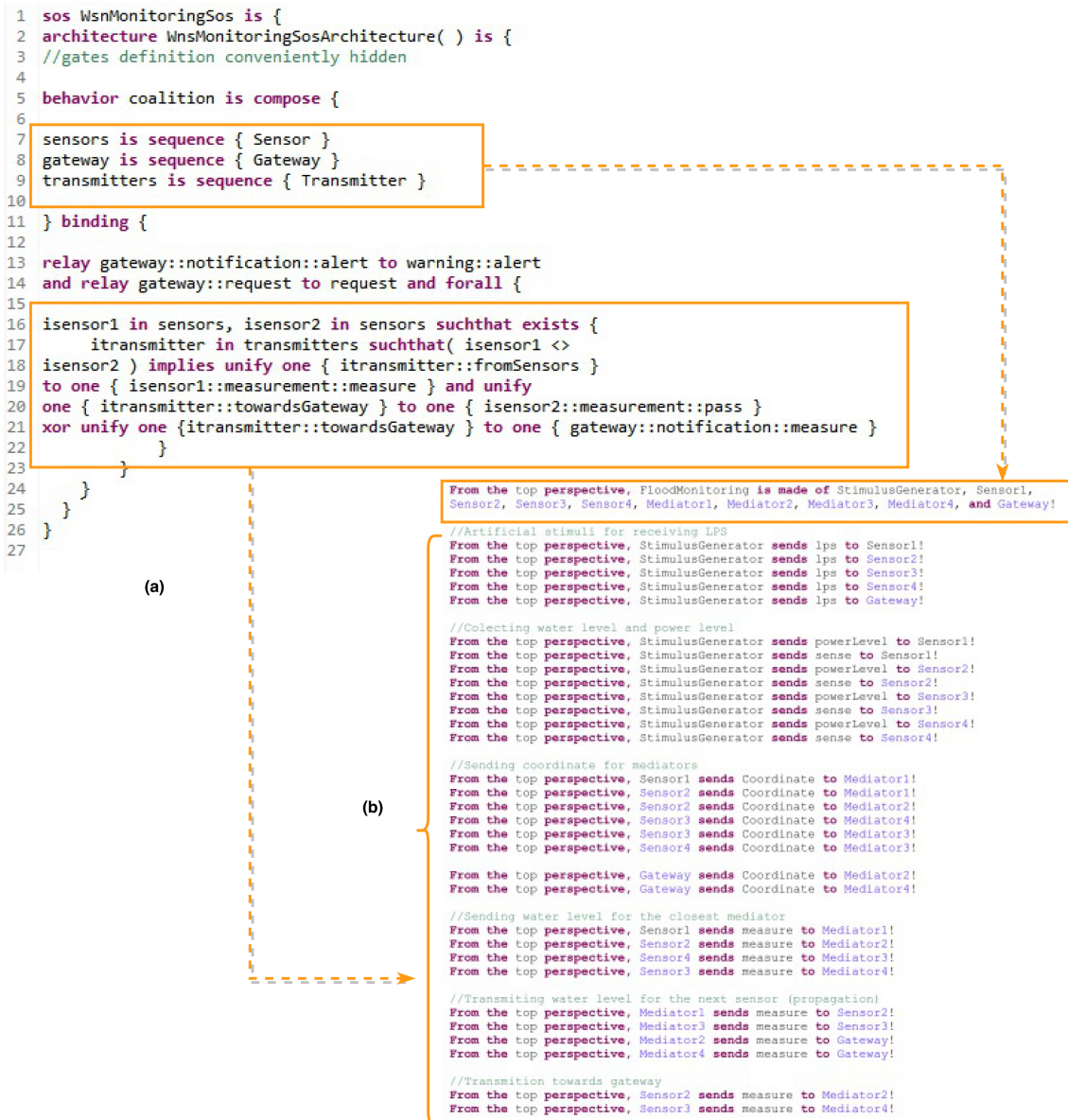
Figure 2.2. A SosADL coalition description mapped to a DEVS simulation model.
